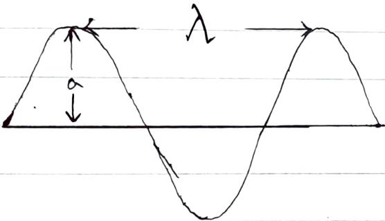
(b) The distance between the peaks of two successive phase is the wavelength 'λ'. The no. of pulses/time is the frequency 'f'.
